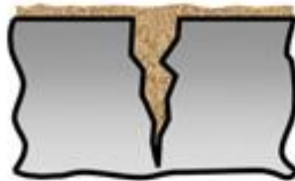
1 Crack filled with dirt
