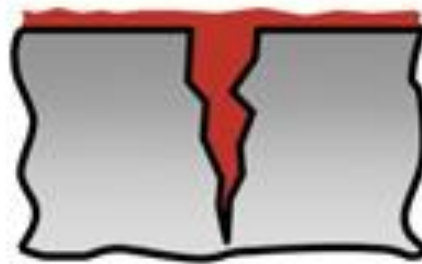
3 Application of penetrant
